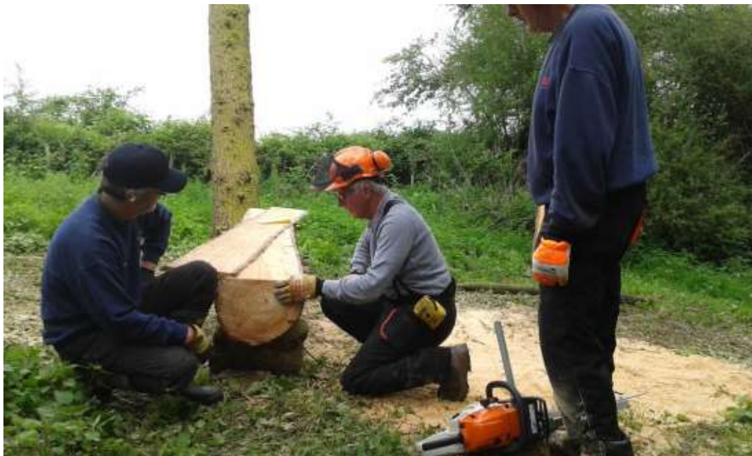
Cutting planks with the milling attachment
